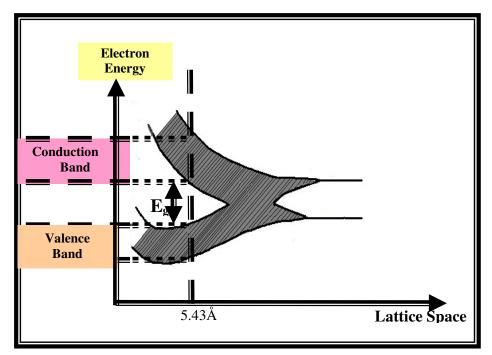
Figure (2-6): Formation of energy bands in silicon lattice crystal by bringing together isolated atoms [75].
