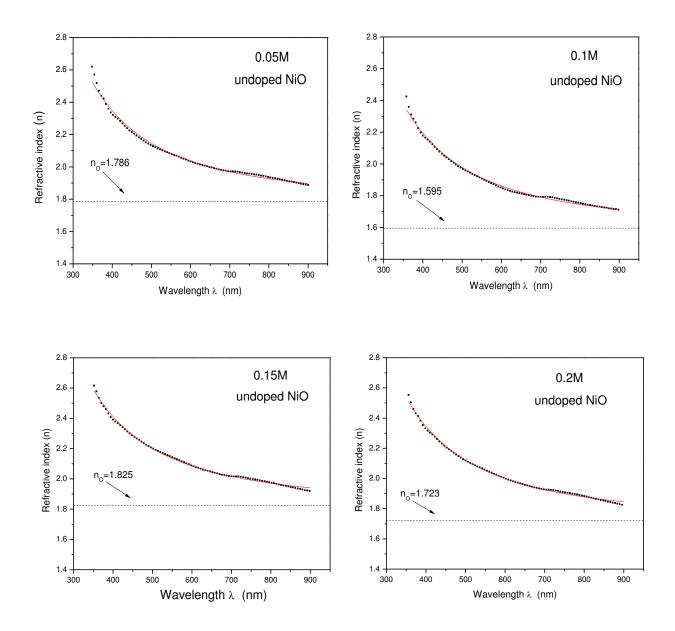
Figure (4-28): Fitting the refractive index data using two terms Cauchy's equation for undoped NiO thin films at different molarities.
