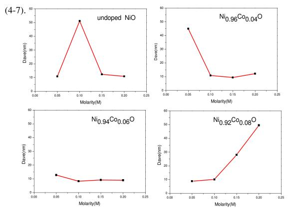
Figure(4-7): The crystallite size  $(D_{av})$  of  $(Ni_{(1-x)}Co_xO)$  thin films, where x = 0, 4, 6 and 8 % at different molarities.
