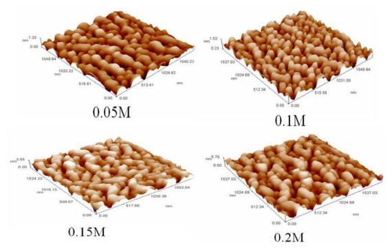
Figure (4-14): 3D AFM images of Ni<sub>0.92</sub>Co<sub>0.08</sub>O thin films at different molarities.
