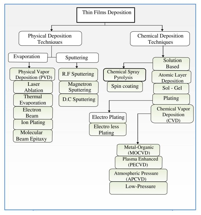
Figure (1-1): Classification of thin film deposition techniques [7].
