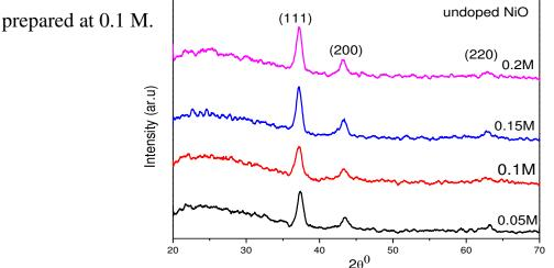
Figure (4-2): XRD patterns of undoped (NiO) thin films at different molarities.
