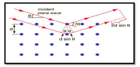
Figure (2-3): Bragg's diffraction [59].
