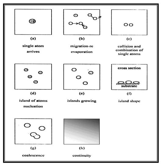
Figure (1-2): Formation Stages of Thin Film [14]
