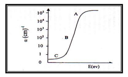
Figure (2-9): The fundamental absorption edge and absorption regions [59].
