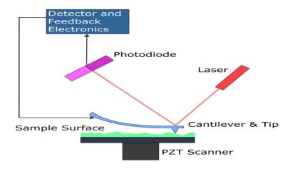
Figure (2-5): Schematic diagram of atomic force microscope [73].
