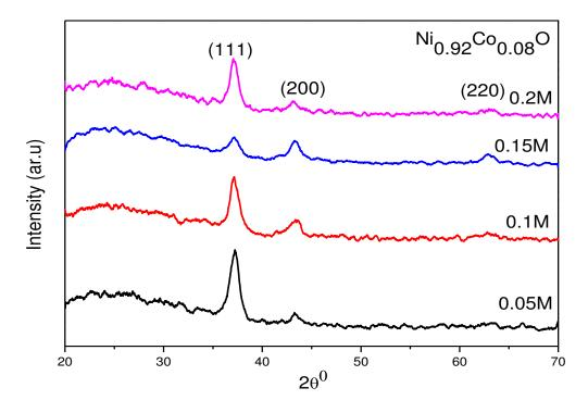
Figure (4-5): XRD pattern of  $(Ni_{0.92}Co_{0.08}O)$  thin films at different molarities.
