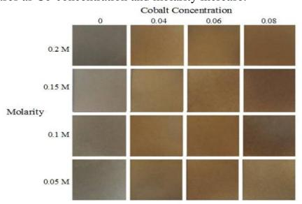
Figure (4-1): Photo image of Nickel-Cobalt Oxide thin films deposited in the present study.
