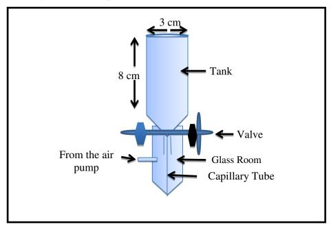
Figure (3-2): Schematic diagram of the spray nozzle.
