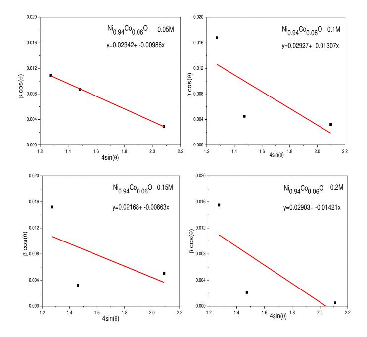
Figure (4-10): The W-H analysis of  $Ni_{0.94}Co_{0.06}O$  thin films at different molarities.
