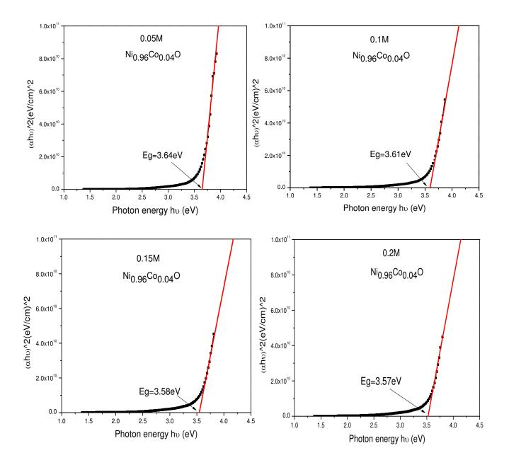
Figure (4-19): The relation between  $(\alpha h \upsilon)^2$  and  $(h \upsilon)$  of Ni<sub>0.96</sub>Co<sub>0.04</sub>O thin films at different molarities.
