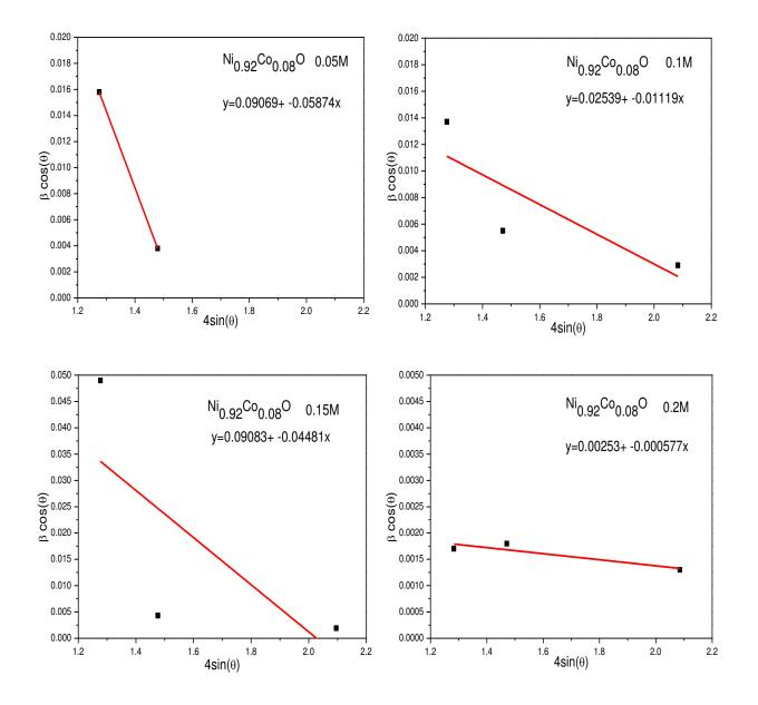
Figure (4-11): The W-H analysis of  $Ni_{0.92}Co_{0.08}O$  thin films at different molarities.
