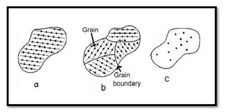
Figure (2-1): Schematics of the general types of materials.a. single crystal, b. polycrystalline and c. amorphous [51].
