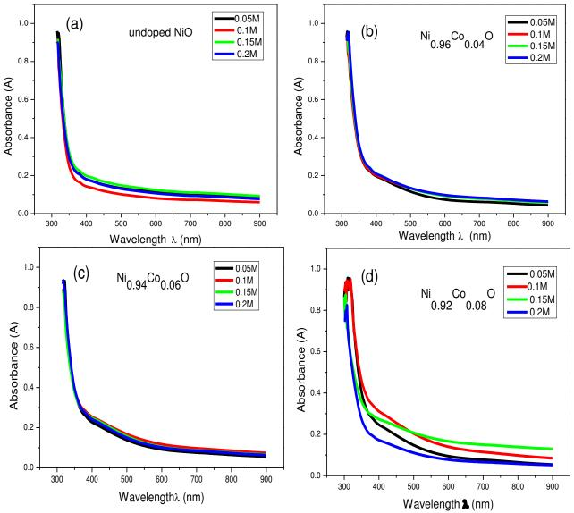
Figure (4-16): Absorbance (A) versus wavelength ( $\lambda$ ) of Nickel-Cobalt Oxide thin films of different molarities.
