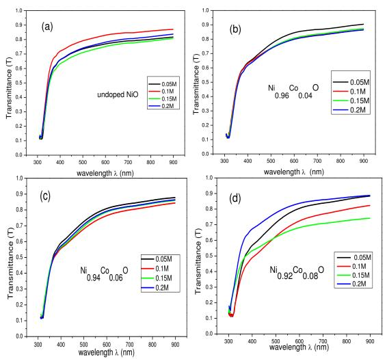
Figure (4-15): Transmittance (T) versus wavelength ( $\lambda$ ) of Nickel-Cobalt Oxide thin films at different molarities.
