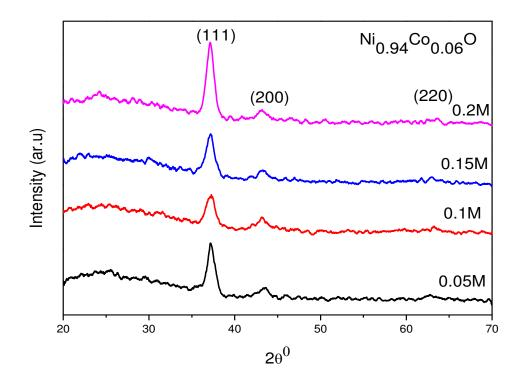
Figure (4-4): XRD patterns of  $(Ni_{0.94}Co_{0.06}O)$  thin films at different molarities.
