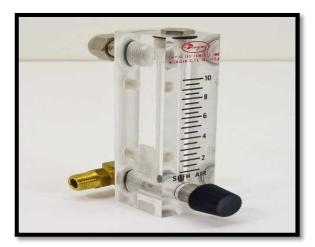
Figure (3-3): Flowmeter device.
