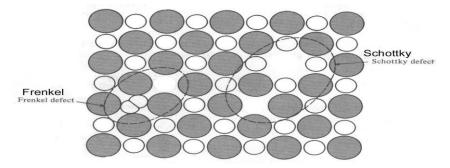
Figure (2-2): Schottky defect and Frenkel defect [55].
