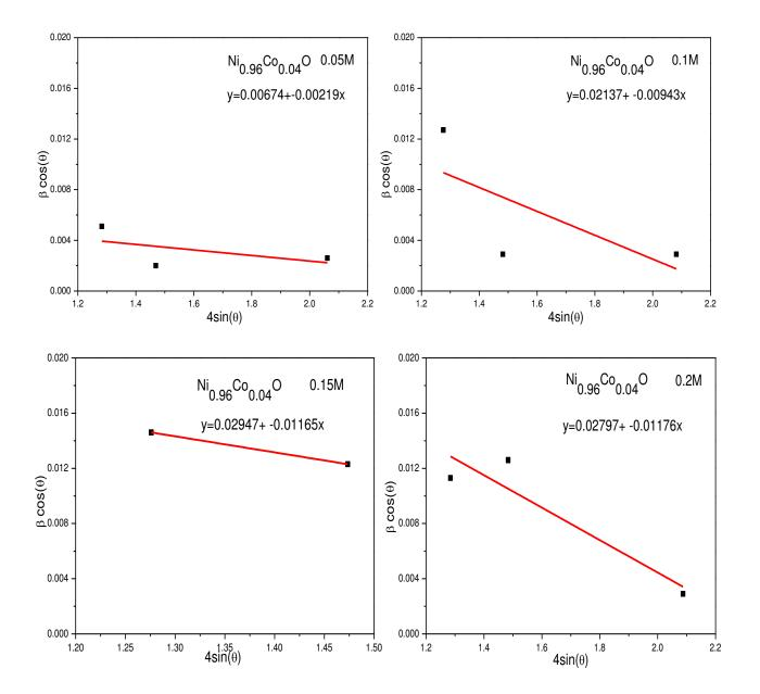
Figure (4-9): The W-H analysis of  $Ni_{0.96}Co_{0.04}O$  thin films at different molarities.
