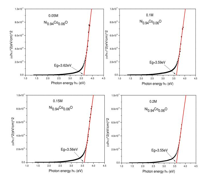
Figure (4-20): The relation between  $(\alpha h \upsilon)^2$  and  $(h \upsilon)$  of Ni<sub>0.94</sub>Co<sub>0.06</sub>O thin films at different molarities.
