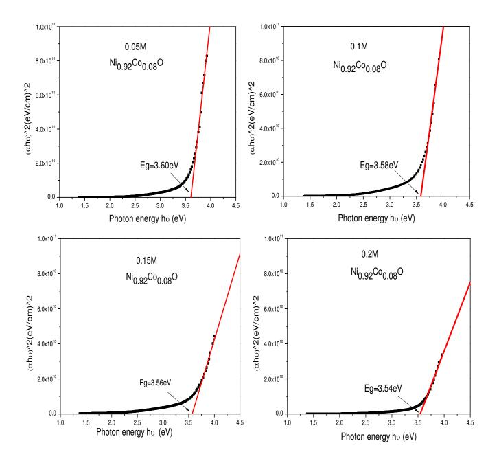
Figure (4-21): The relation between  $(\alpha h \upsilon)^2$  and  $(h \upsilon)$  of  $Ni_{0.92}Co_{0.08}O$  thin films at different molarities.
