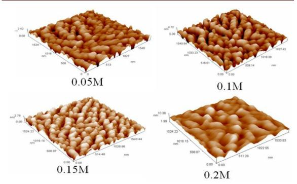
Figure (4-12): 3D AFM images of undoped NiO thin films at different molarities.
