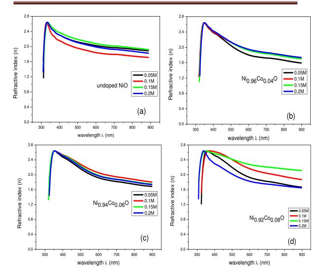
Figure (4-27): The relation between the refractive index and wavelength for Nickel-Cobalt Oxide thin films for different molarities.
