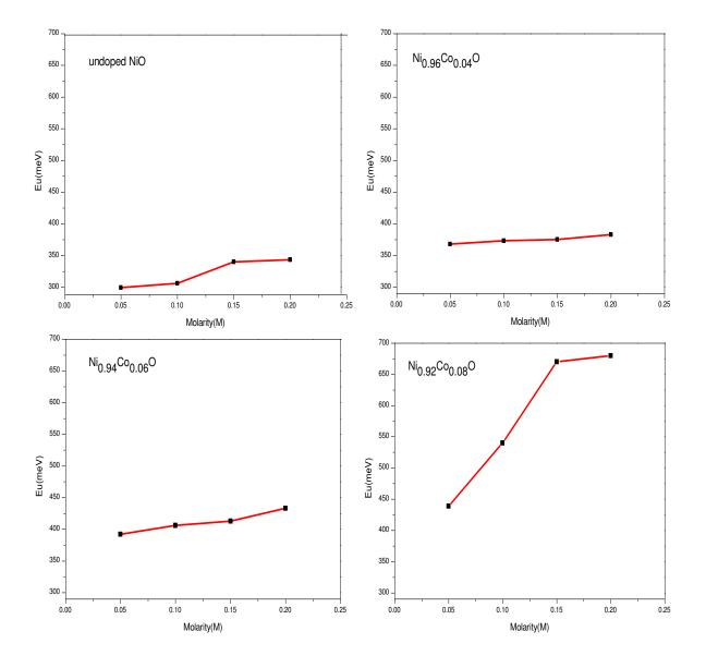
Figure (4-25): The variation of urbach energy as a function of molarity for Nickel- Cobalt Oxide thin films.
