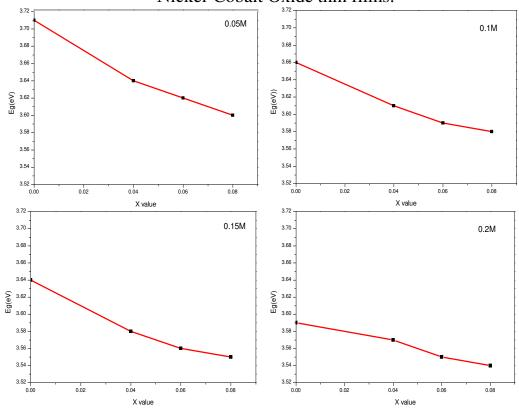
Figure (4-23): The variation of energy gap as a function of concentration for Nickel-Cobalt Oxide thin films.
