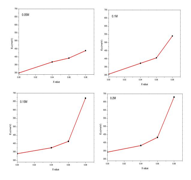
Figure (4-26): The variation of urbach energy as a function of concentration for Nickel-Cobalt Oxide thin films.
