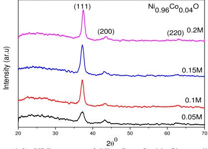
Figure: (4-3): XRD patterns of  $(Ni_{0.96}Co_{0.04}O)$  thin films at different molarities.
