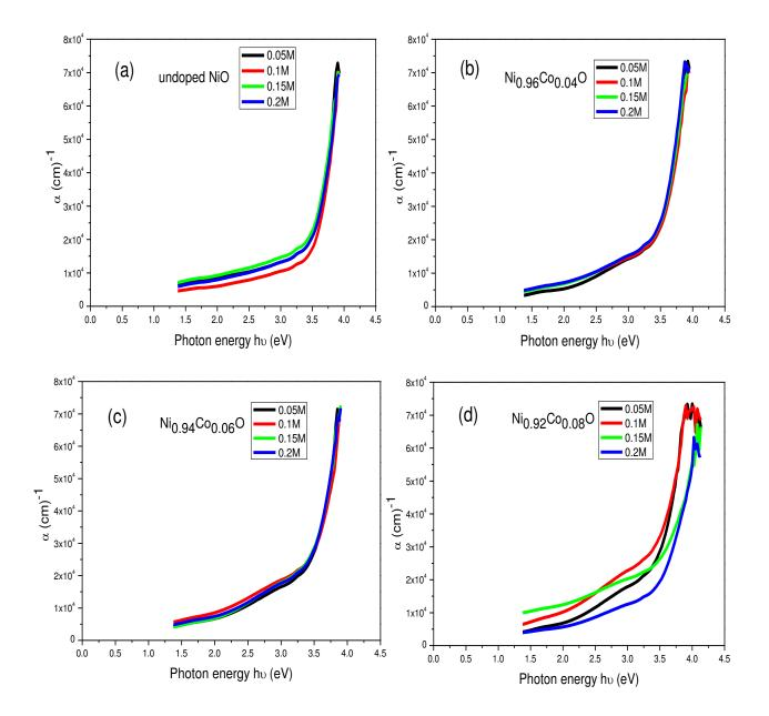
Figure (4-17): The relation between absorption coefficient and photon energy of Nickel-Cobalt Oxide thin films at different molarities.
