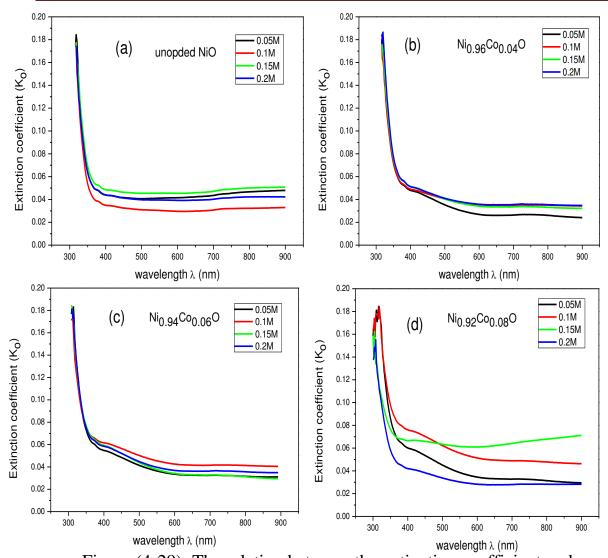
Figure (4-29): The relation between the extinction coefficient and wavelength for Nickel-Cobalt Oxide thin films at different molarities.
