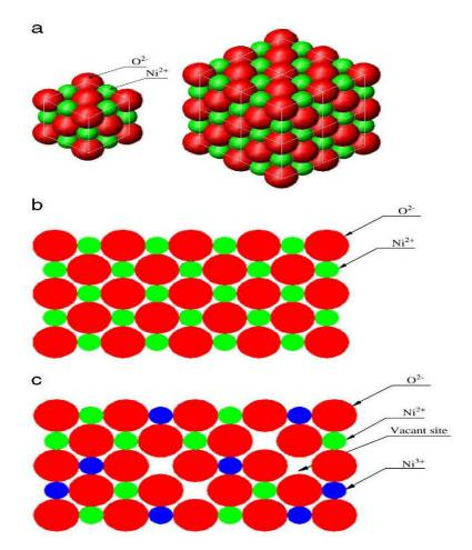
Figure (1-3): Structure of nickel oxide. [16]
