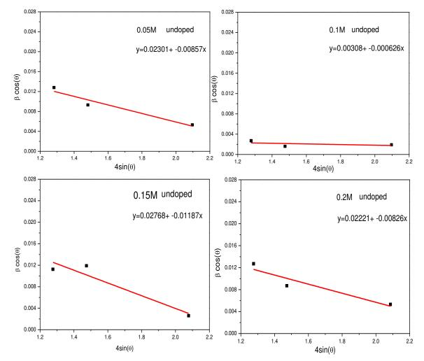
Figure (4-8): The W-H analysis of undoped NiO thin films at different molarities.
