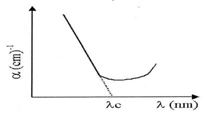
Figure (2-8): Fundamental absorption edge of crystal semiconductor [79].
