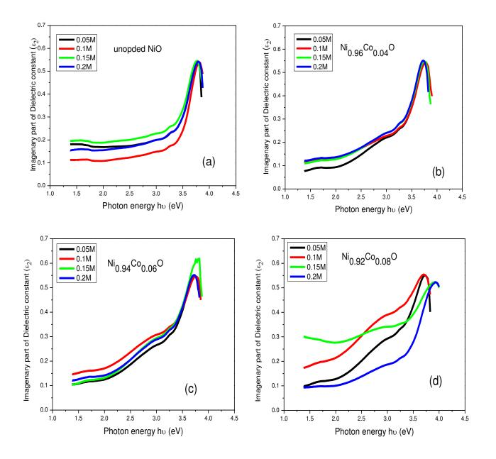
Figure (4-31): The relation between the imaginary part of dielectric constant ( $\epsilon_2$ ) and photon energy for Nickel-Cobalt Oxide thin films at different molarities.
