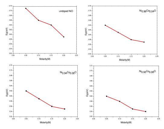
Figure (4-22): The variation of energy gap as a function of molarity for Nickel-Cobalt Oxide thin films.
